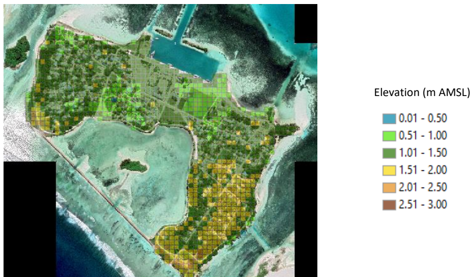
Figure 221: Elevation data assigned for SWB modelling - GDh. Faresmaathoda Island
