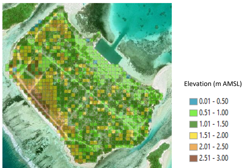
Figure 190: Elevation data assigned for SWB modelling - GDh. Rathafandhoo Island
