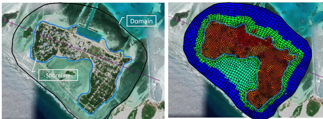
Figure 225: Model boundaries and model mesh - GDh. Faresmaathoda island
