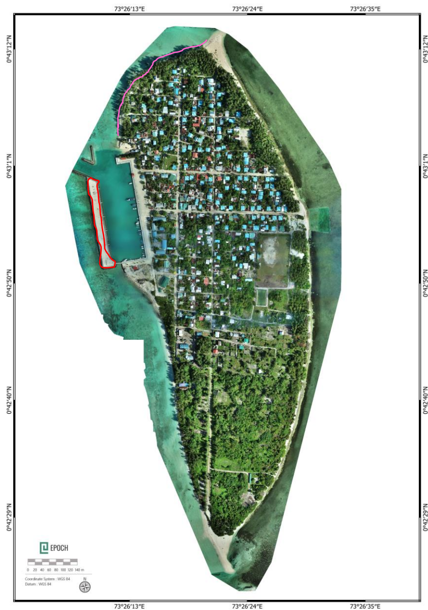
Figure 41 GA. Maamendhoo Orthomosaic illustrating the eroding area (pink), detached breakwater (red)
