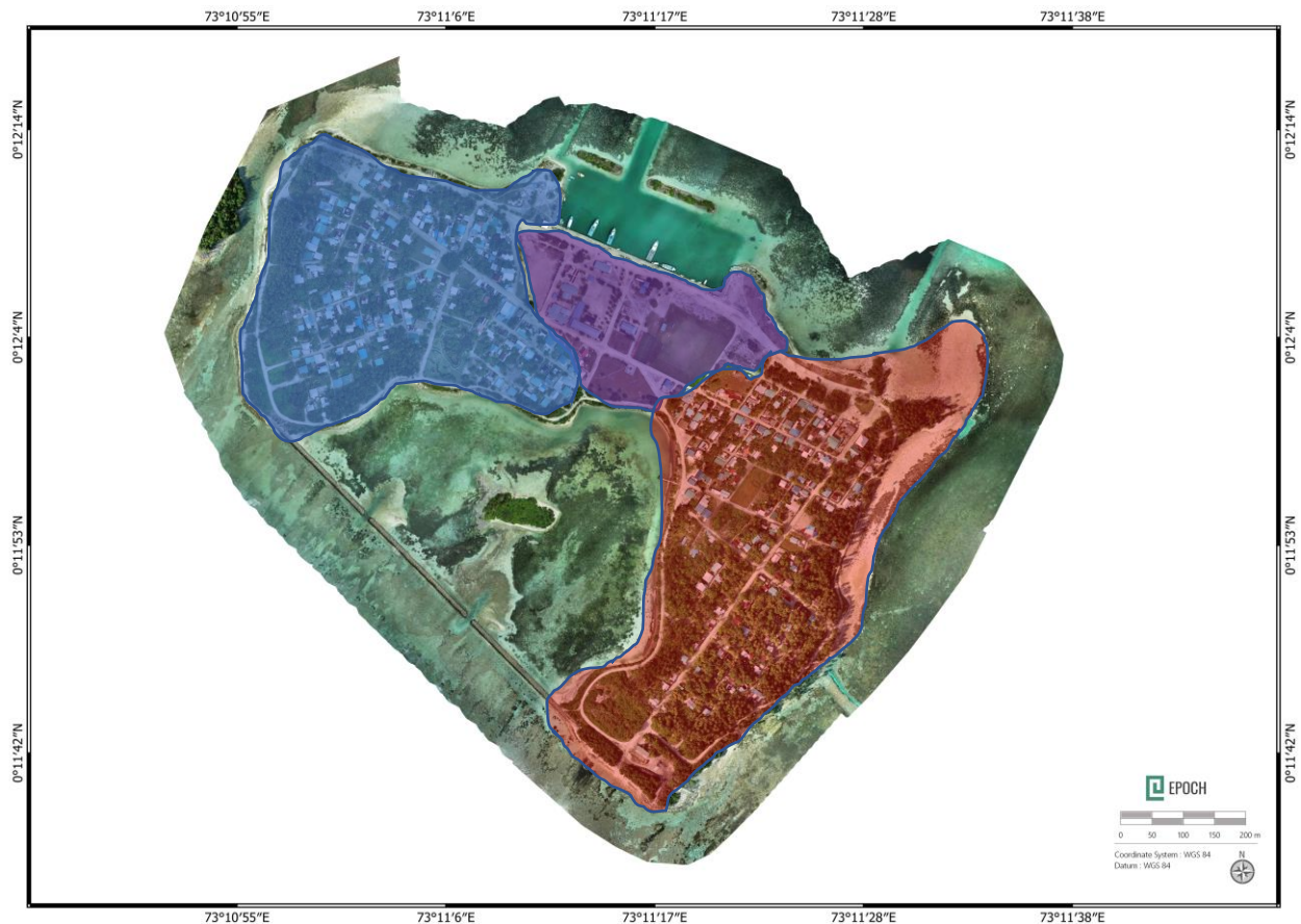
Figure 203 Orthomosaic of GDh. Faresmaathoda. Original Maathodaa Island is shown in blue, Original Fares Island is shown in red and reclaimed area is shown in purple
