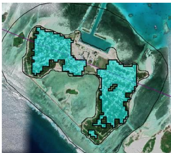
Figure 227: Pumping region at SUTRA model - GDh. Faresmaathoda island
