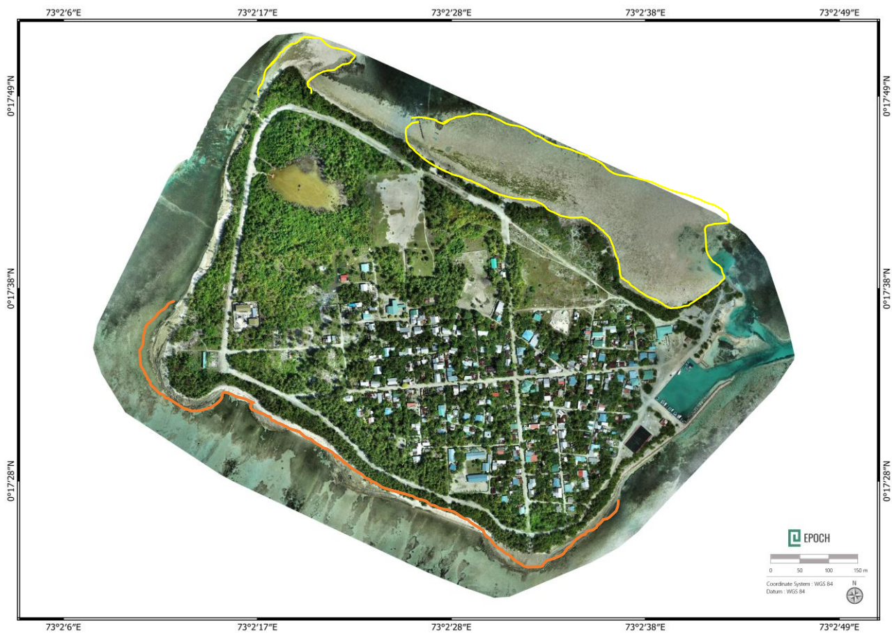
Figure 140 Orthomosaic preview of Nadella with windward region with large gravel sized sediment (orange) and fanned out sediment that are exposed during low tide (yellow)
