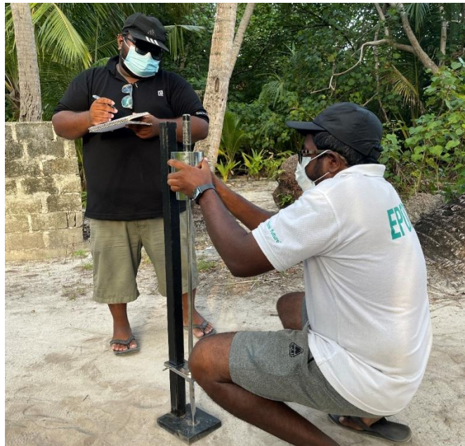
Figure 21: Dynamic Cone Penetrometer Testing on-site
