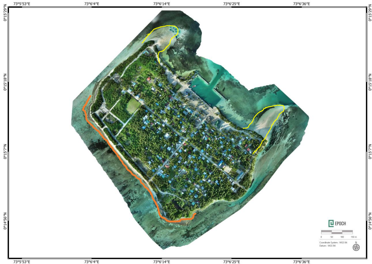
Figure 172 Orthomosaic generated for GDh. Rathafandhoo. Windward region with large gravel sized sediment (orange) and fanned out sediment that are exposed during low tide (yellow)
