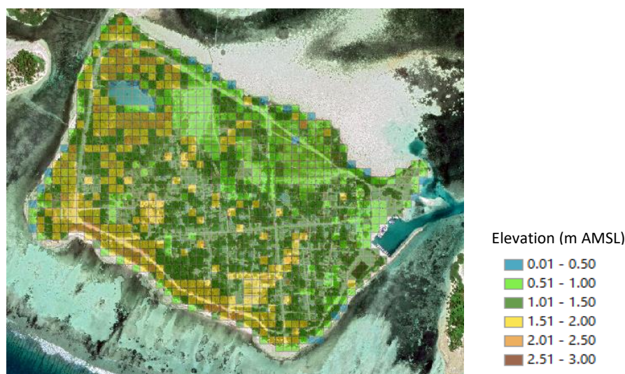
Figure 158: Elevation data assigned for SWB modelling - Nadella Island
